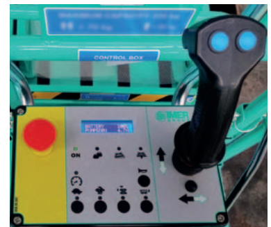
Control panel on the platform with capacitive buttons: simplicity and safety of use
